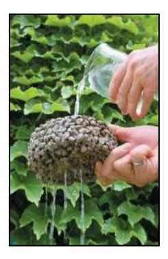
The photo left shows water poured onto and through pervious concrete. Typical flow rates through pervious concrete are about 8 inches per minute, much faster than for most lawns.
