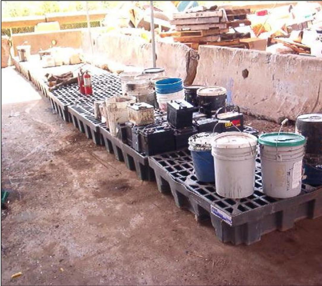
**Secondary containment should be used to prevent materials from contaminating stormwater.**
